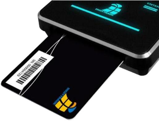
If an invalid or defective smart card is inserted in the smart card slot the “ERROR”-LED will flash three times and illuminates then permanently red. In that case please contact DIGITTRADE.
