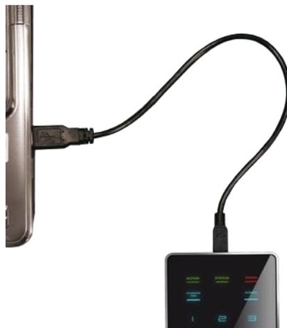
**Note:** Do not use the DIGITTRADE HS256 S3 via a buspowered USB hub or extension cable and ensure it has enough power.
